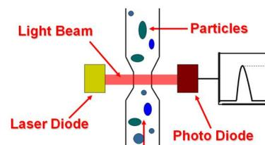
The amplitude of the pulse is then compared to the instruments calibration curve to determine the approximate size of the particle. The output of the sensor is a stream of pulses of varying amplitude, each corresponding to a particle. This type of device is known as a light blocking or light extinction particle counter.
