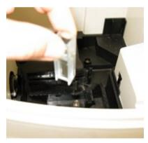
This method is based upon the transmission of light. A specific wavelength of light (around 360nm in the case of chlorine dioxide) is passed through a cuvette containing the sample, and the transmission/absorption is measured.
